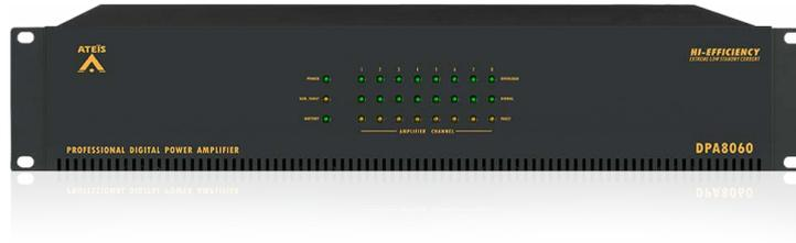
The DPA is a digital power amplifier with extremely low power consumption (0.2W per channel) during standby mode, and high amplification efficiency of 90%. A four-step DIP switch can be configured to enable/disable the function of standby mode (power-save mode) when powered by AC mains; to request the LEDs on the front panel to comply to EN 54-16; and to enable/disable the battery monitoring.
